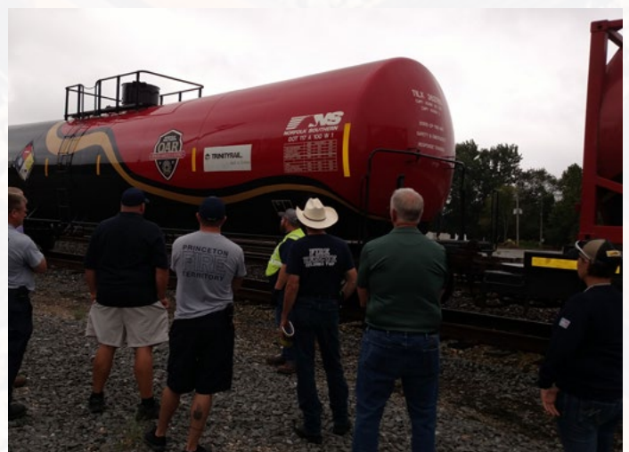
Brian Shanks (Norfolk Southern) explains the DOT 117A100W1 general purpose tank car. ■
