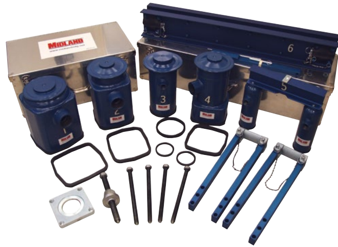
Midland B-240/B-243 Emergency Response Kit consists of a toolbox containing a broad range of tools and replacement parts; cover cans of five different sizes that are used to cap a leaking valve or fitting, along with corresponding gaskets; and a bridge that is used to secure a cover can to the railcar's manway cover plate.
